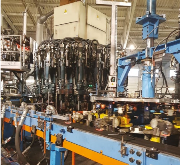
Olivotto's OGT 4.0 approach applied to a press and blow automatic forming line.
